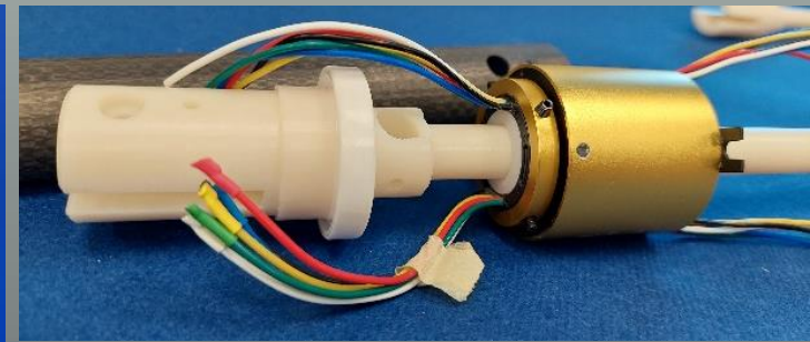
Accura 25® 3D-printed parts with 0.2 mm tolerance (required machining)
