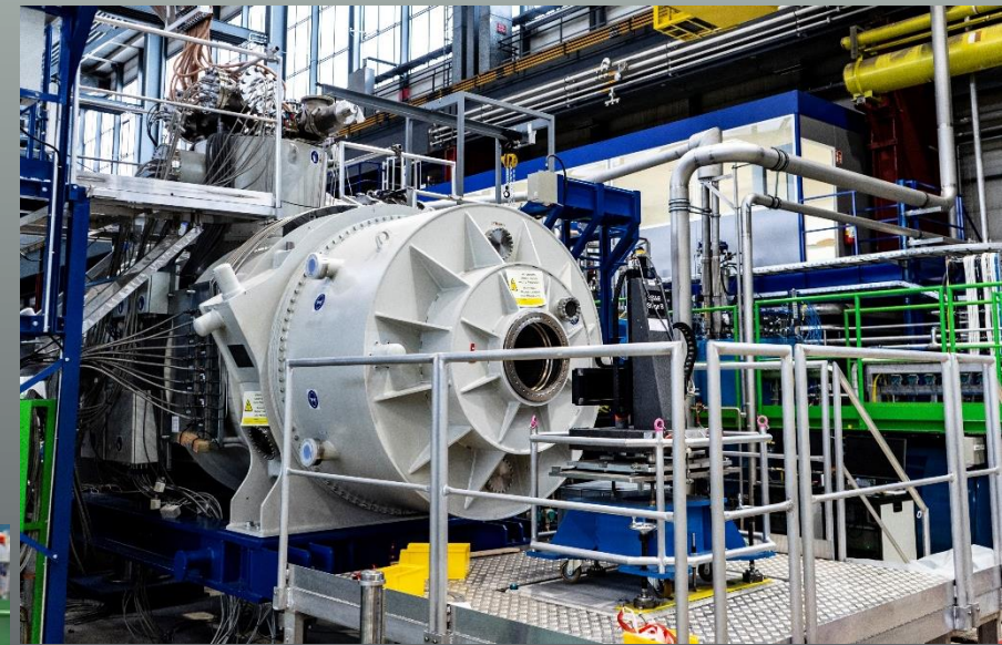
First short multiples being tested with SSW
