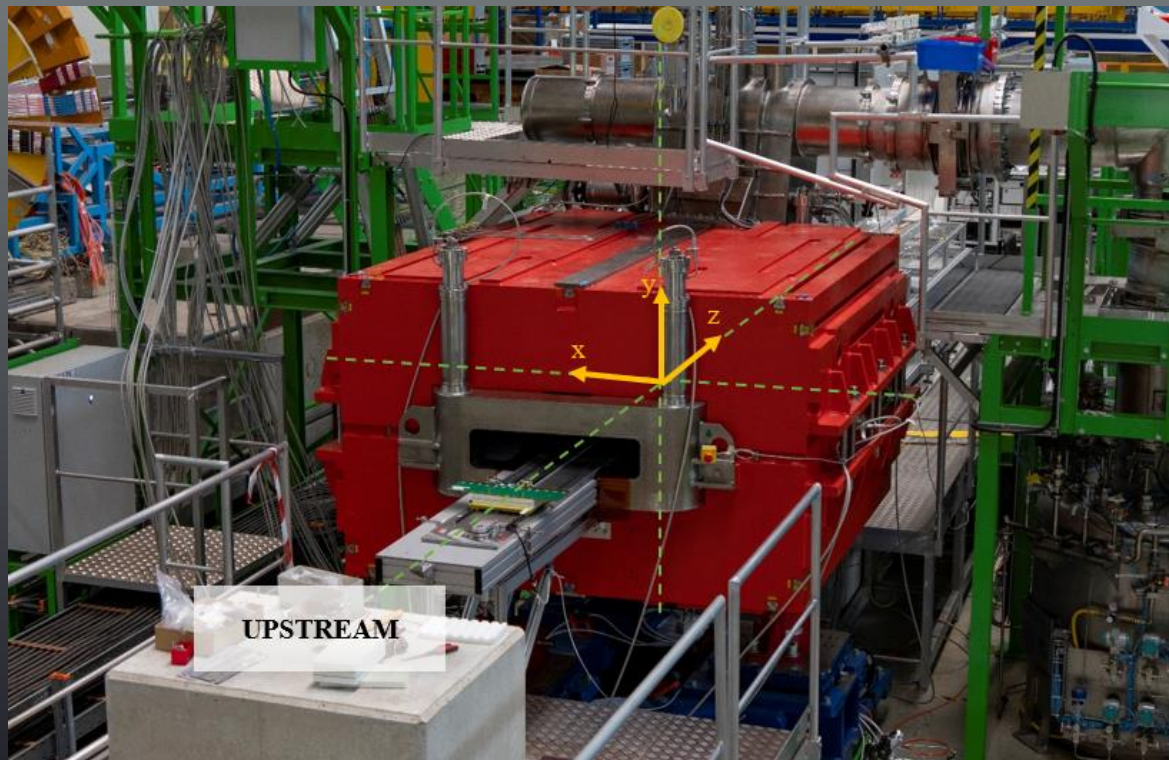
First main bending dipole being tested with translating fluxmeter
