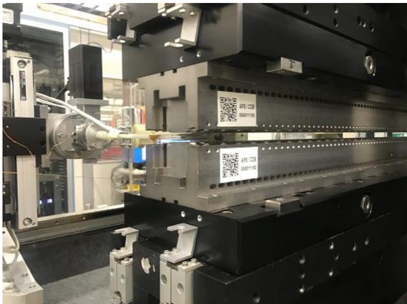
Photograph of the reference undulator APS25#4. Configuration: Hybrid planar Period length: 25 mm Total length: 2.4 m
