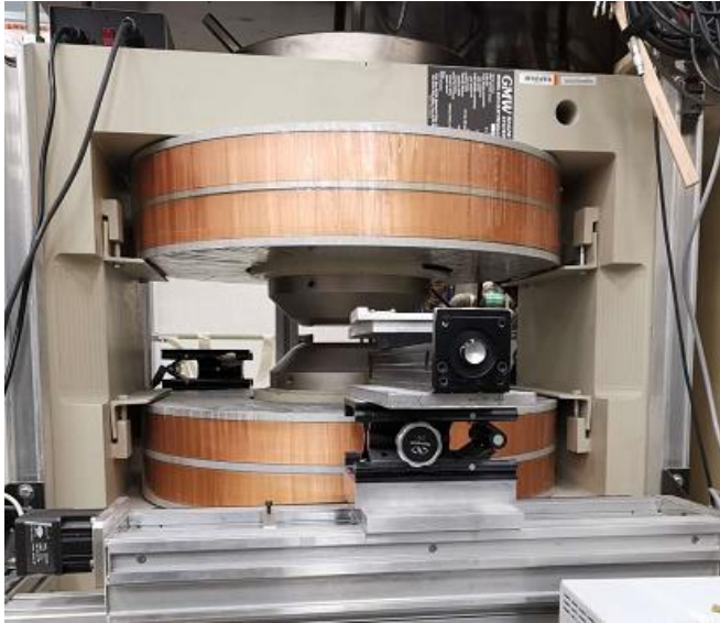
Standard (reference) dipole magnet used for Hall sensor calibration in the Magnetic Measurement lab (MM1) at the Advanced Photon Source (APS).
