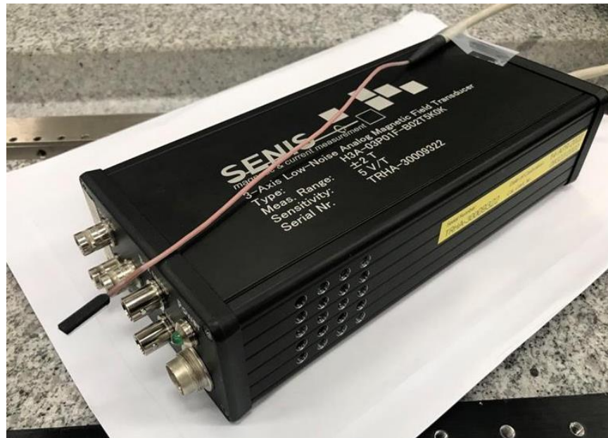
Photograph of the Senis 2-axis high-precision Hall sensor and transducer. Sensitivity: 5V/T
