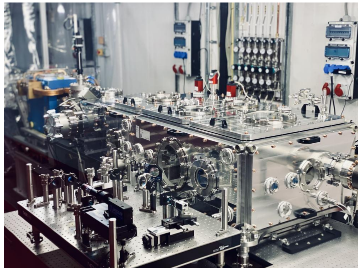
Figure 1 : Vacuum-Chamber of the KALDERA-Plasma-Cell [1].
