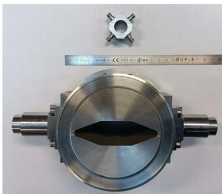
BPM prototypes for SOLEIL (bottom) and SOLEIL II (top)
