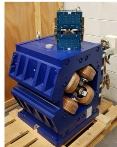
Permanent magnet quadrupole prototype (top) for SOLEILII and Electromagnet quadrupole for SOLEIL
