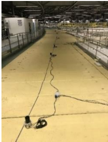
Neutron monitor on the Storage ring roof Distributed by Radosys (Hungary)
