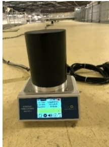
Neutron monitor on the Storage ring roof Distributed by Radosys (Hungary)
